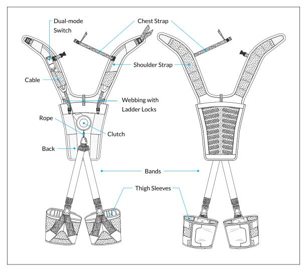
The Apex's Shoulder Straps and Back components are worn like a backpack. The Thigh Sleeves are worn around the thighs in a manner similar to athletic equipment like thigh pads or thigh compression garments.
