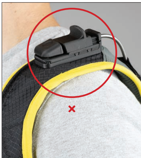
Figure 21: Male Straps Adjusted Incorrectly. Straps too loose. Note height of Switch.
